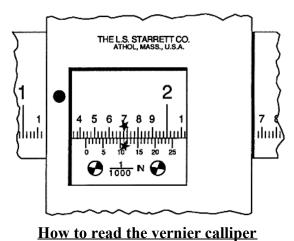
Read the number of full inches that show from zero on the main scale to zero on the vernier. In the figure, this would be 1.000 inch.
